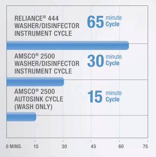
Electric heat, non-vented, double door units are compared.
